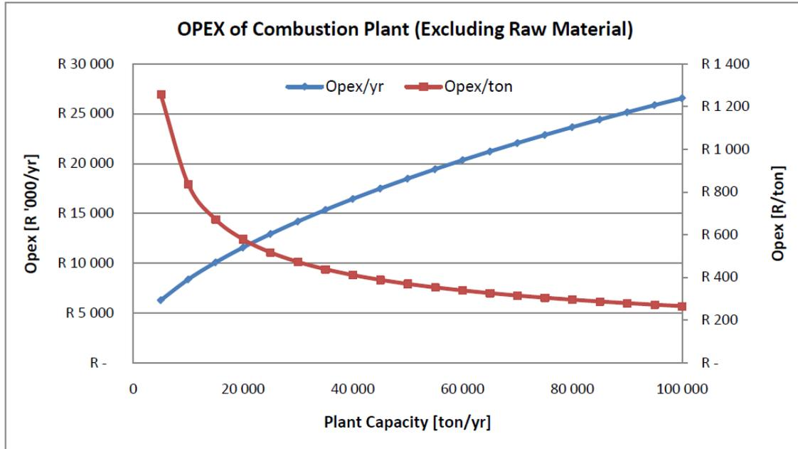
Figure 4: Operating cost of a combustion plant
