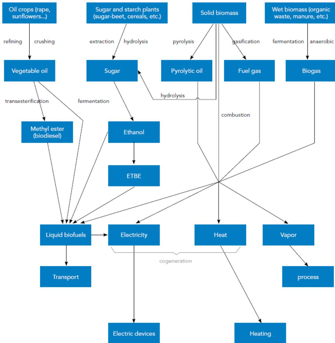
Figure 2: Biomass conversion flow (Kimble, et al., 2008).
